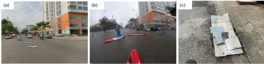
Fig. 1. Daily conditions in the Thac Gian-Vinh Trung area: (a) dry-season conditions extracted from Google Earth, (b) localized flooding during heavy rainfall (photo by Anh Tuan Dang, December 9, 2018) and (c) a street inlet covered by boards to block sewer odors (photo captured by researchers, November 27, 2025)
